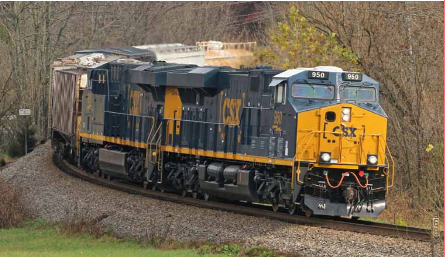
Two brand new CSX General Electric-made ES44AC locomotives with the CSX new “boxcar” logo move southbound train Q696-03 at Slant, Va., on Nov. 4, 2011. The units each pack 4,400 hp each and weigh about 216 tons each. Chris Starnes
