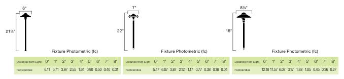
DESIGN PRO LED PATH & SPREAD LOW VOLTAGE
